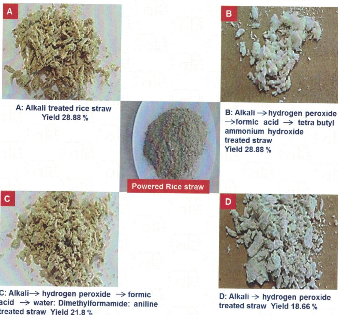
Figure 6. Form and yields of cellulose from powdered rice straw through different processes.
